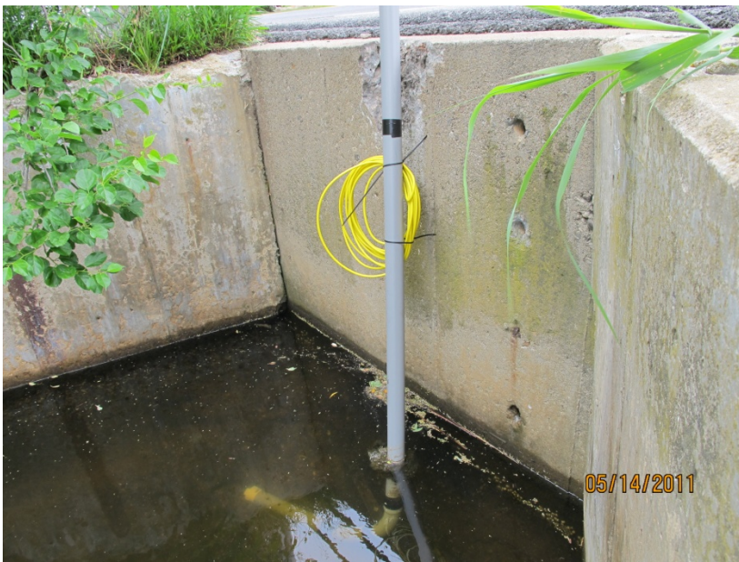
Above: Upstream culvert data logger. Below: Downstream culvert data logger.
